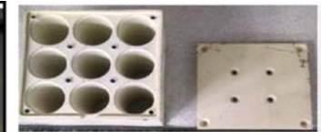
Figure 8: Intumescent material before fire
