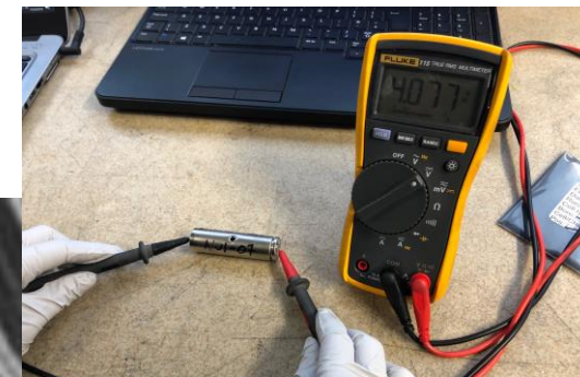
Cell with nail-hole is still working.
