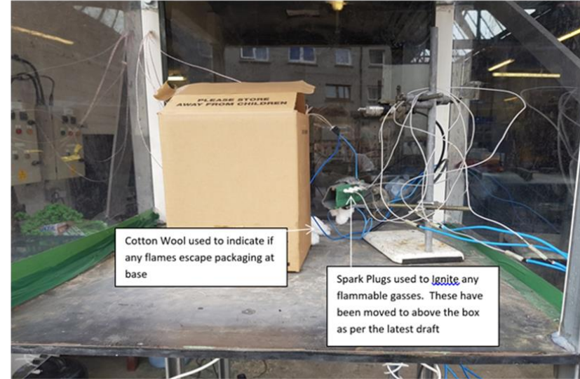
Setup of spark ignitors and cheesecloth
