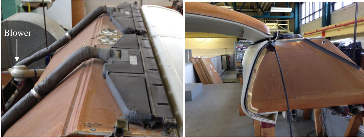
a) ECS diffuser ducts, blower. Bin doors open b) Ceiling panel added. Bin doors closed
