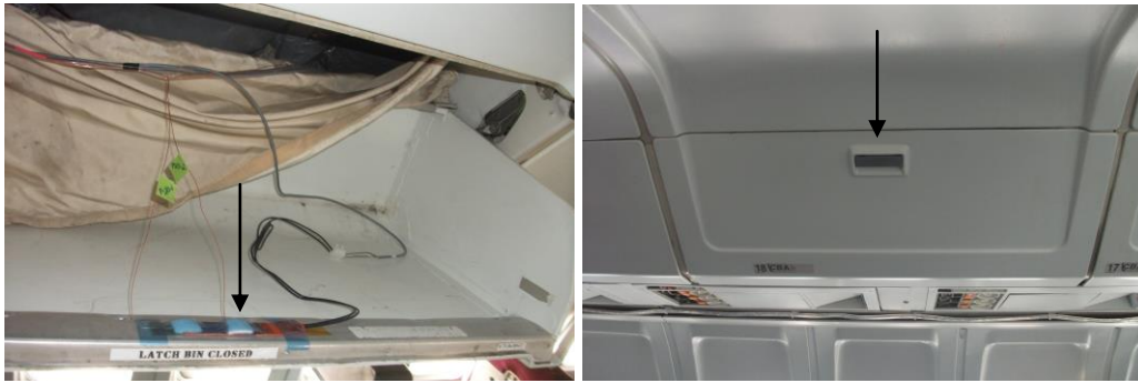
Fig. 16. P1 heater and TC installation in port Bin 18.
