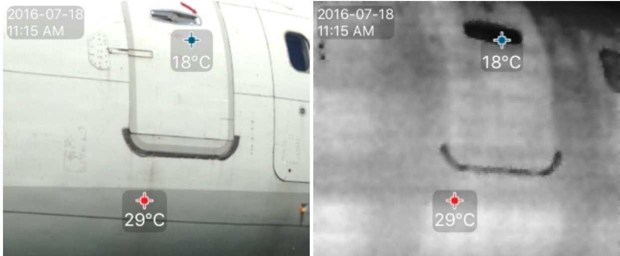
Fig. 13. SEEK visual and thermal pair of the ERS aircraft exterior at the L1 door.
