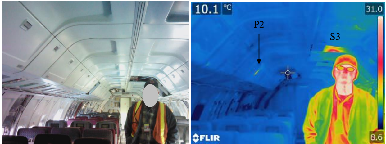
Fig. 23. Visual and Thermal image pair, from aft. Sites P2 and S3 marked.
