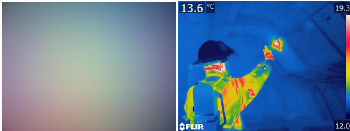
Fig. 12. FLIR T650sc Visual and Thermal image pair, in fog.
