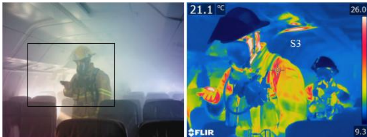
Fig. 10. FLIR T650sc visual and thermal image pair of heat source in ceiling panel. Note second firefighter obscured by fog.
