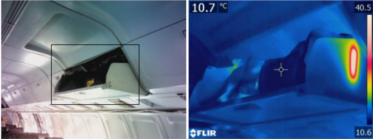
a) FLIR T650sc Visual and Thermal image pair
