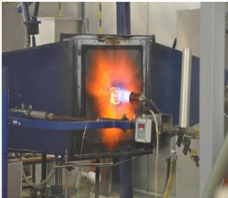
Flame exposure Test (5min)
