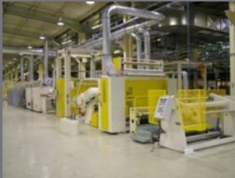
4. High pressure water jets entangle the fibres
