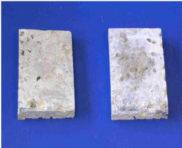
+ ZE41 – Poor corrosion performance
