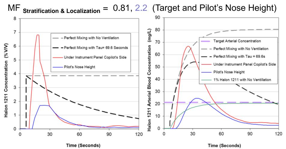
Based on data from 1984 Report, Fig 6, Test 4
