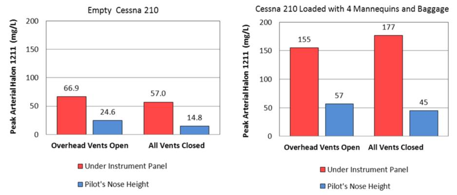
Halon 1211 arterial blood concentrations for under the instrument panel are underestimated for the loaded aircraft, as the gaseous concentrations were off-scale.
