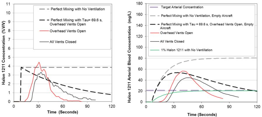
• Halon 1211 perfect mixing gas and arterial blood concentrations are underestimated for the loaded aircraft, as the free space volume and air change time are unknown.
