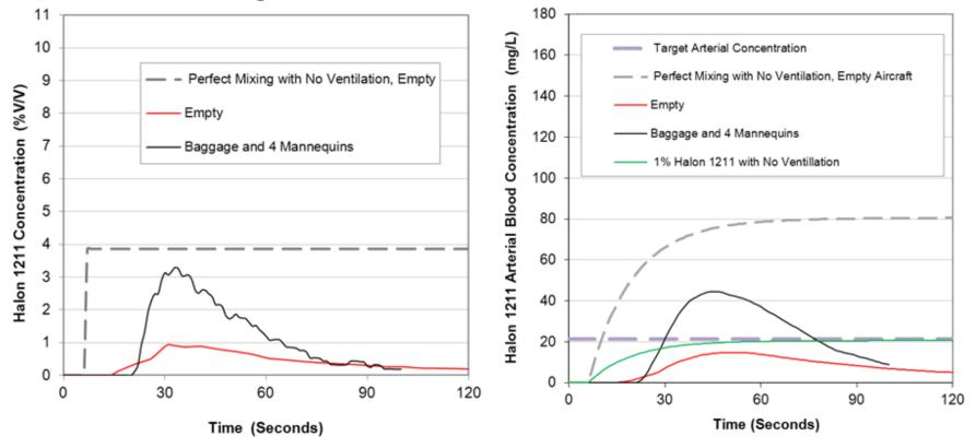
• Perfect mixing Halon 1211 gas and arterial concentrations are higher for the loaded aircraft: Free space volume and air change time are unknown
