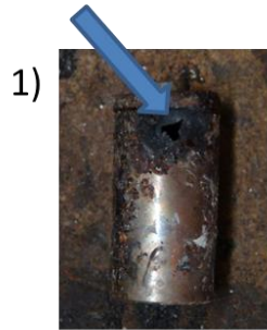
Vent holes were in alternate locations.
