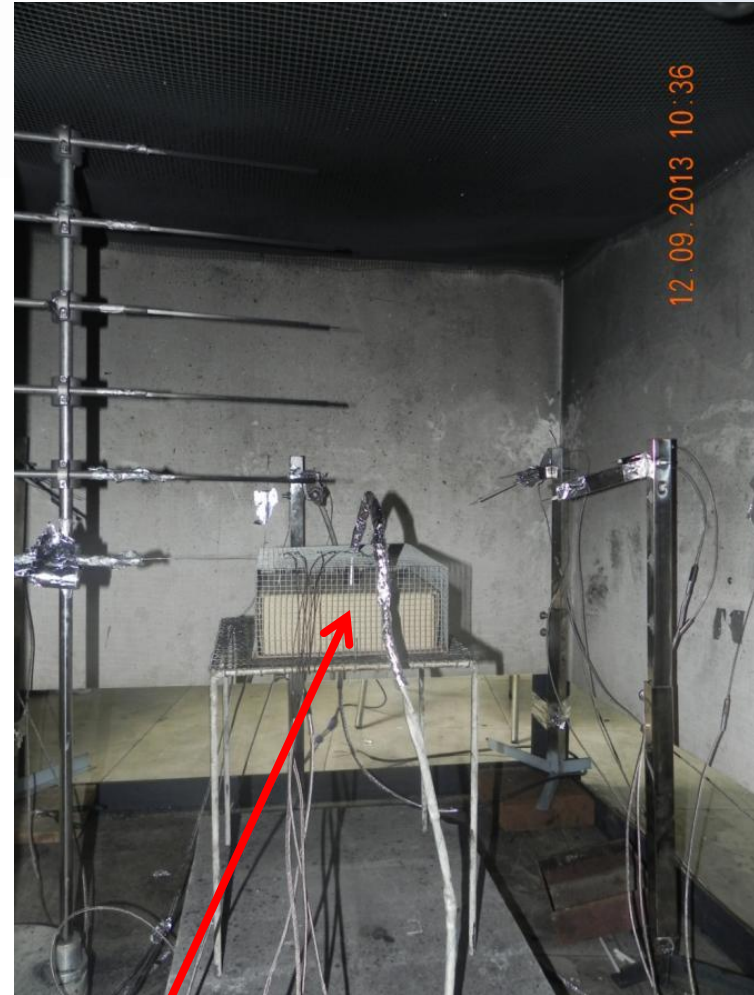
Propagation thermal runaway test: Electric heater
