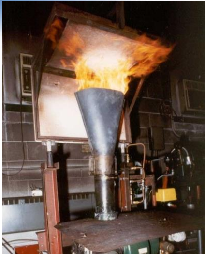
Oil burner (cargo liner criteria test)
