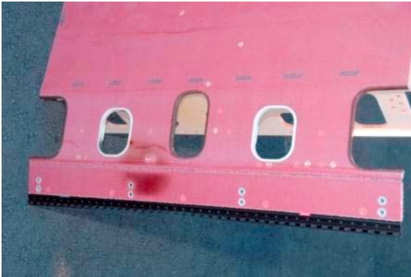
Inserts along an edge for trim attachment
