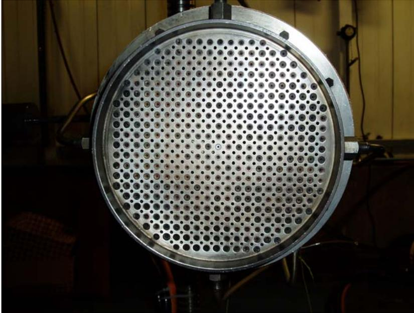
Burner exit plane, 373 large holes – fuel and primary air,
