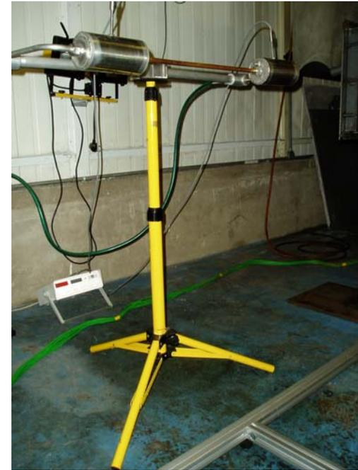
Measurements of heat flux using a continuous water flow calorimeter
