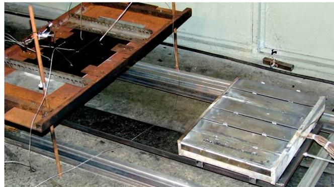
► The composite test sample is 10 cm above the horizontal radiant panel
