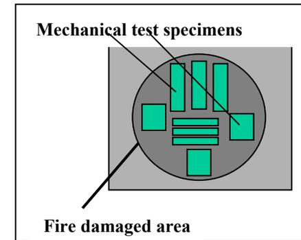
➔ The loss of mechanical properties is already very significant after only 25s of exposure to the fire source
