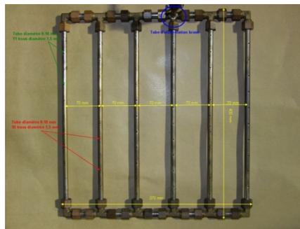
A propane fire source has been designed **on the basis of the FAA foam block fire source characteristics**, assuming that these characteristics are representative of a declared hidden fire :
