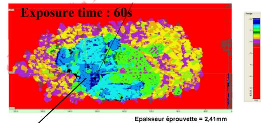
80% of the thickness is delaminated after 1 mn of exposure
