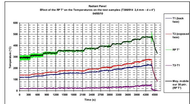
► The next step was to find the setting  $T^\circ$  of the radiant panel which generates surface temperatures of the composite material close to the resin glass transition  $T^\circ$  (190 / 200°C):
