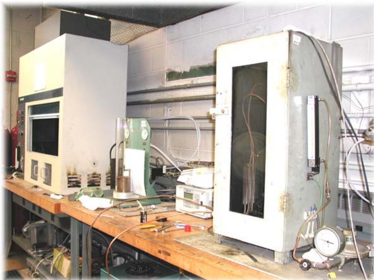
Vertical Bunsen Burner Test Apparatus (FAR 25.853 or Handbook)
