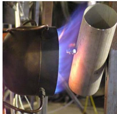
➤ Tube and bolt (simulating the critical part)
