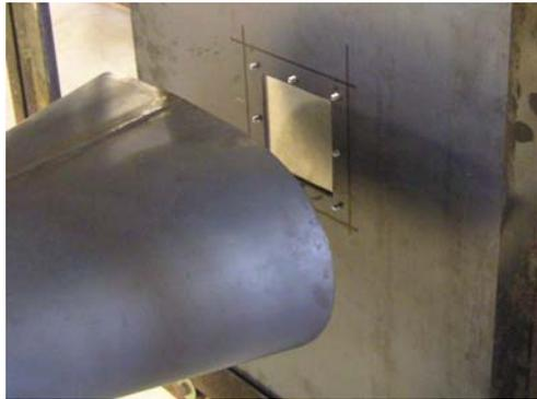
A 1.2mm aluminium plate is fitted behind a 3mm steel plate, simulating a critical area to be tested
