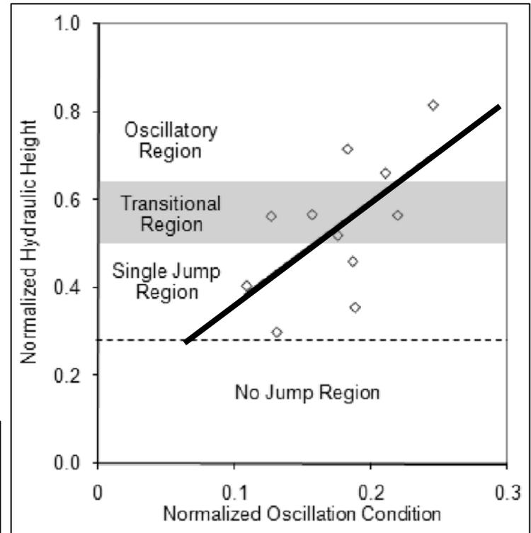
$$Normalized\ Oscillation\ Condition = \frac{y_{max}}{h_0} * \frac{f}{f_0}$$
