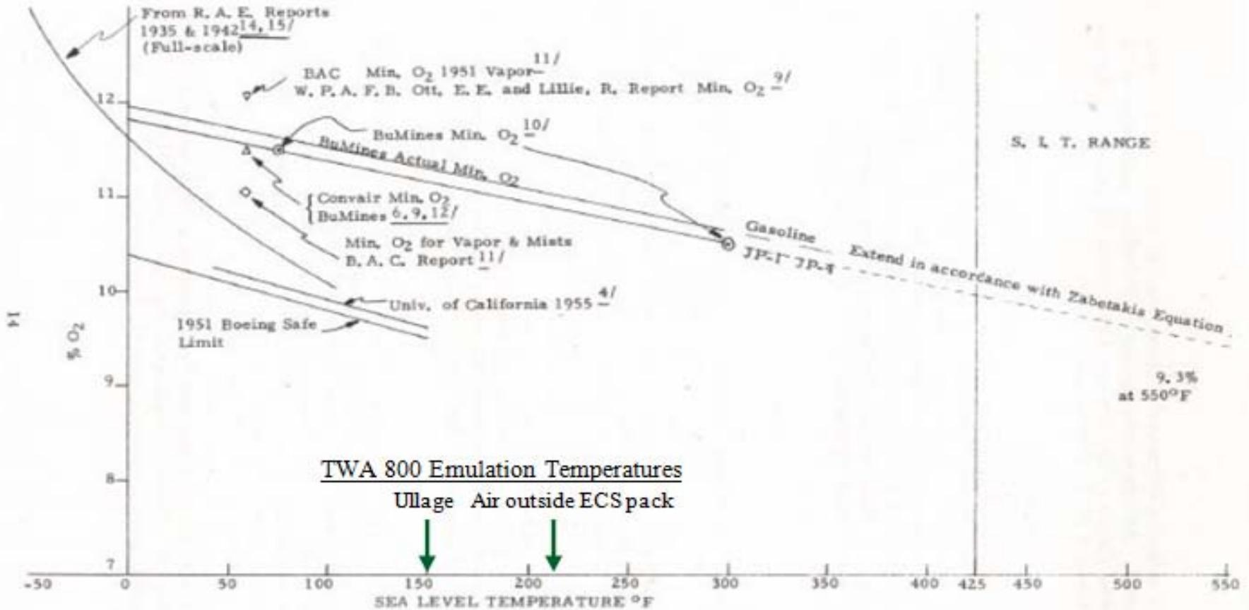
FIG. 9 COMPOSITE CHART OF INERTING REQUIREMENTS AS PLOTTED FROM LITERATURE SEARCH
