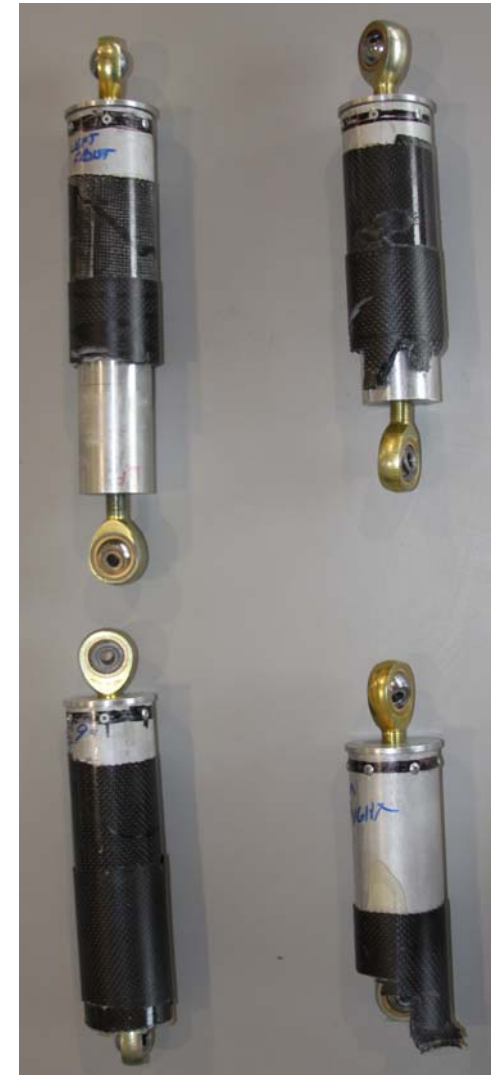
Post-test photo of shock struts following Test #1
