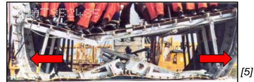
flattening of lower fuselage shell:
