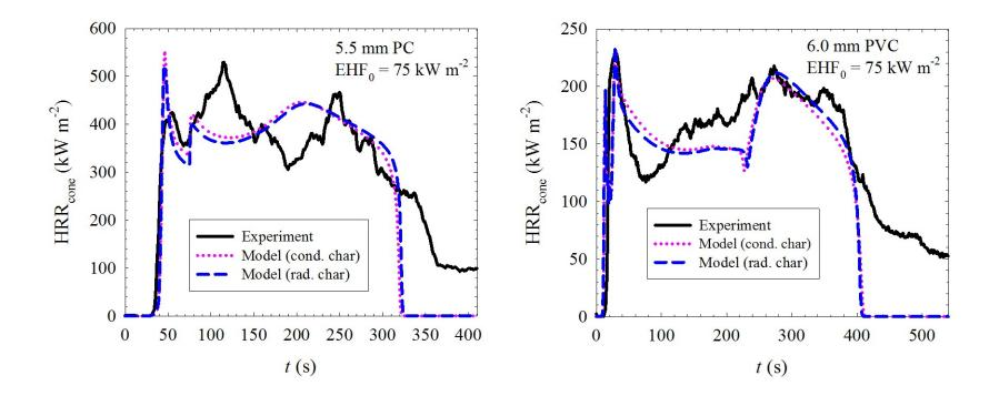
If the char layer is a stack of graphitic plates, which exchange energy via radiation, the layer thermal barrier efficiency depends only on the number of plates in this layer.
