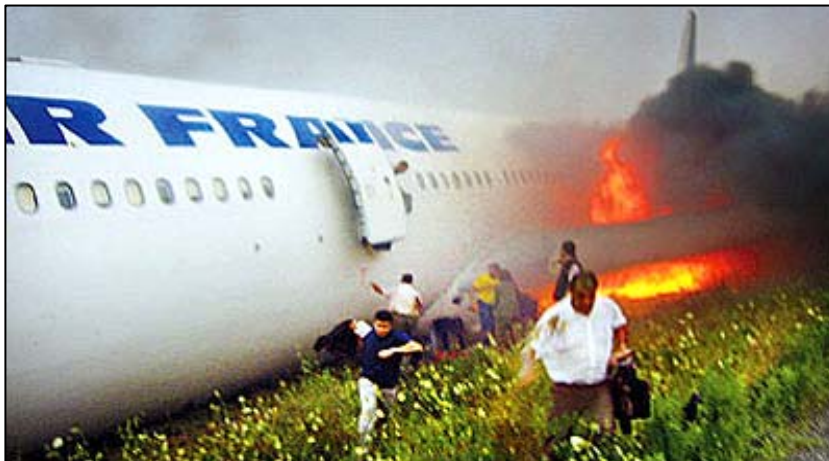
Toronto, Canada, August 2, 2005: Flame retardants were credited with increasing escape times for all 309 passengers from this jet, which was ultimately completely consumed by fire.
