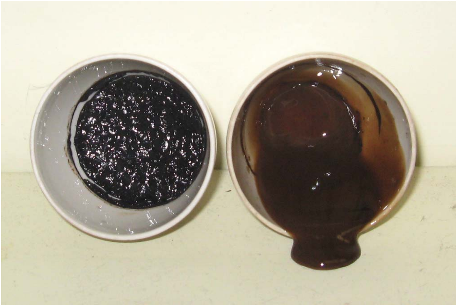
CNFs dispersion (left) and OM-clay (right) in polyol after annealing 10 min at 350°C
