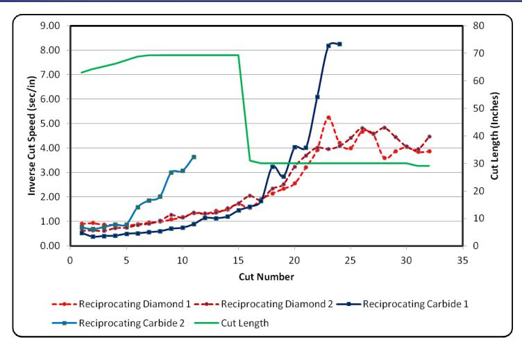
Diamond blade still sharp and capable of cutting additional materials. Carbide blades were dull and could not cut more than two sheets. Each sheet represented 127 linear feet of cutting.
