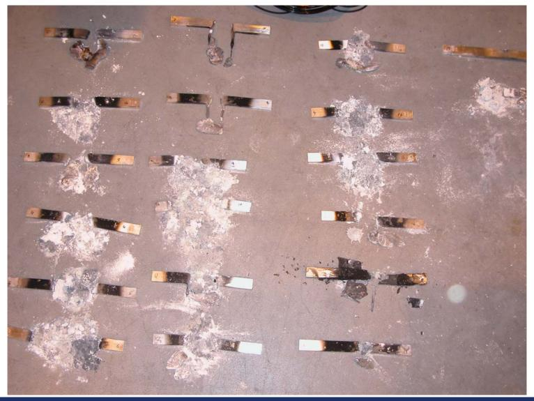
Magnesium Bar Samples Post-Test
