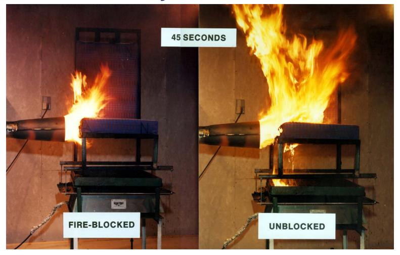
Performance test based on results of full-scale tests
