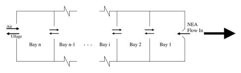
Next, modified model to split flow to several bays and vent flow from several bays using flight test data for ratios
