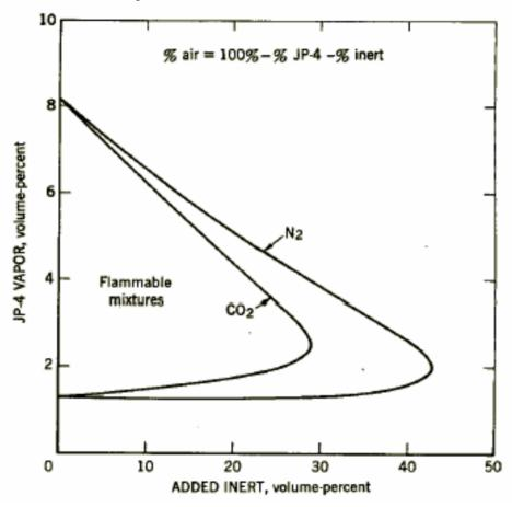
Flammability limits of JP-4 vapor-CO<sub>2</sub>-Air and JP-4 vapor-N<sub>2</sub>-Air Mixtures at 27° C and atmospheric pressure. (Zabetakis, 1965)
