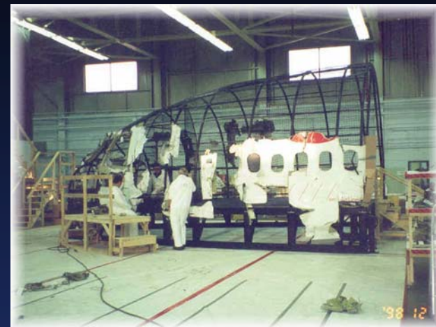
SwissAir MD-11 Accident Investigation Reconstruction, 1998
