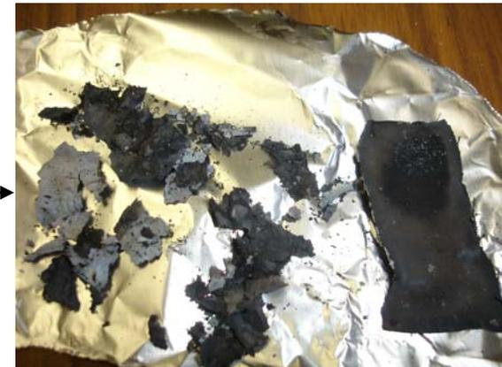
Burning of A12-TiO<sub>2</sub> coated camouflage fabric
