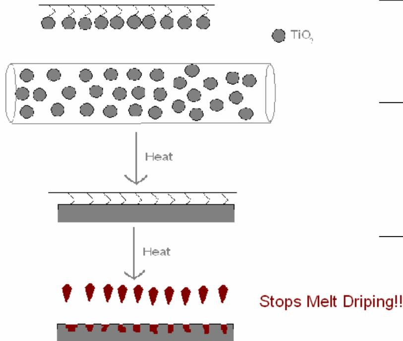
→ **Covalent attachment of metal oxide nanoparticles (TiO<sub>2</sub>) to FR polymer**
