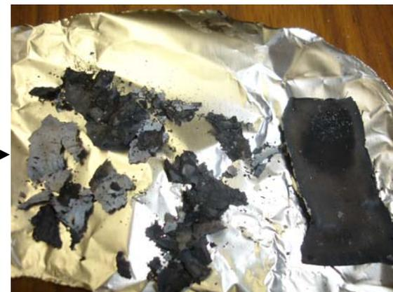
Burning of A12-TiO<sub>2</sub> coated camouflage fabric
