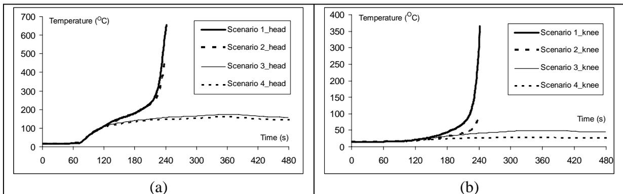
Figure 5: Predicted temperatures at (a) head height and (b) knee height in Zone 25
