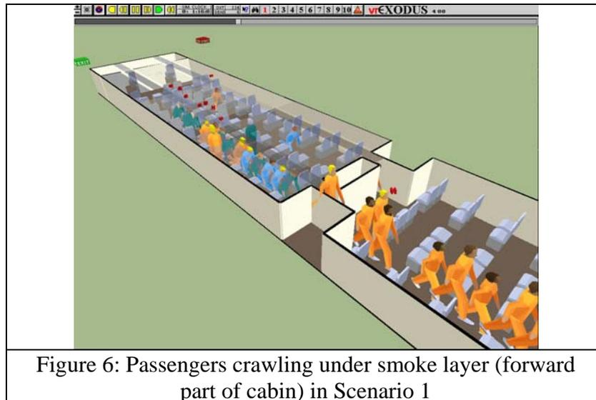
Figure 6: Passengers crawling under smoke layer (forward part of cabin) in Scenario 1
