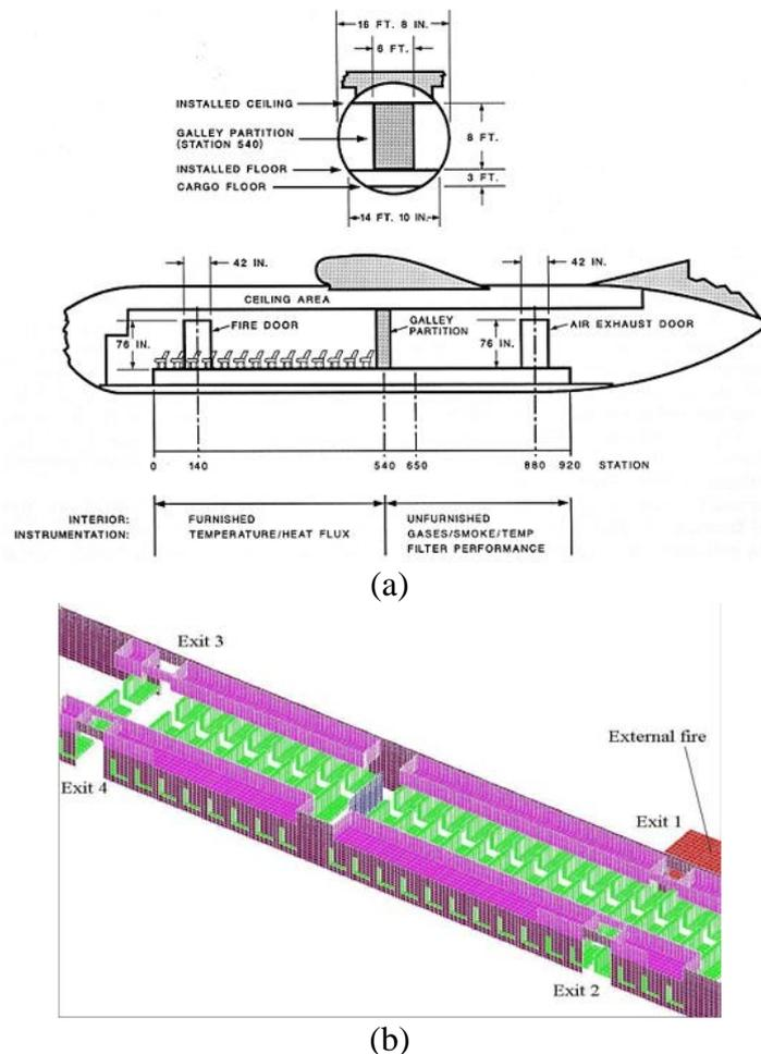
Figure 1: C-133 geometry (a) full-scale test facility (reproduced from [3]); (b) configuration used in fire simulation
