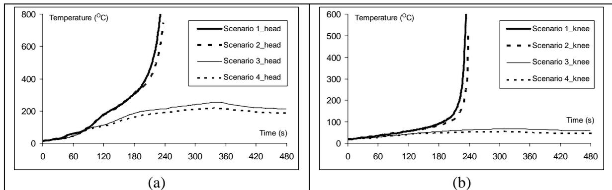
Figure 3: Predicted temperatures at (a) head height and (b) knee height in Zone 8
