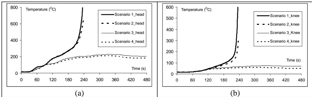
Figure 4: Predicted temperatures at (a) head height and (b) knee height in Zone 18
