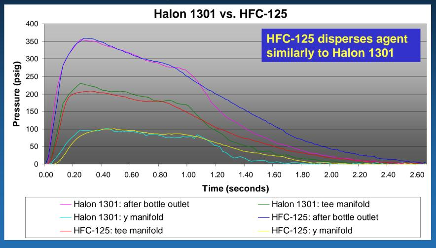
Based on discharge test results, HFC-125 is a viable simulant for Halon 1301
