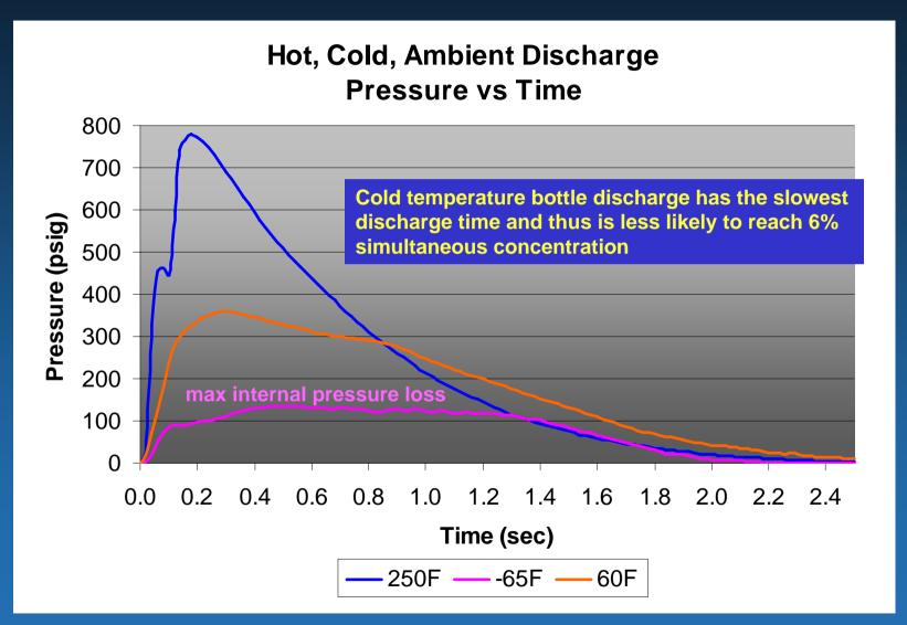
Ground test to be conducted with cold-soaked bottle
