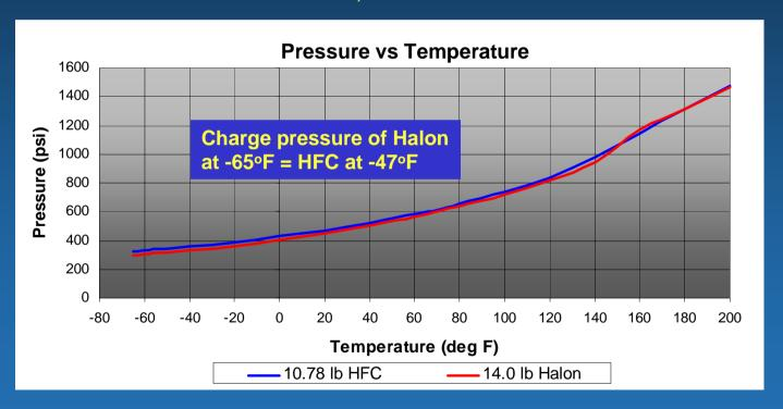
HFC-125 at -47°F is equivalent to Halon 1301 at -65°F
