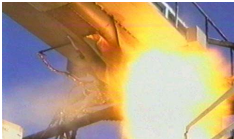
Ballistically induced fire in the fuselage dry bay of an aircraft detected and extinguished < 200 milliseconds
