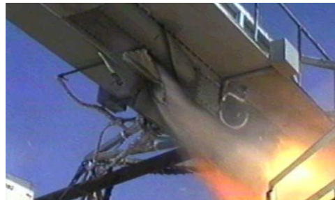
Ballistically induced fire in the fuselage dry bay of an aircraft detected and extinguished < 200 milliseconds
