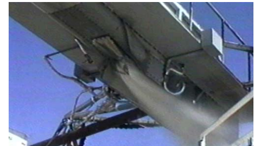
Ballistically induced fire in the fuselage dry bay of an aircraft detected and extinguished < 200 milliseconds
