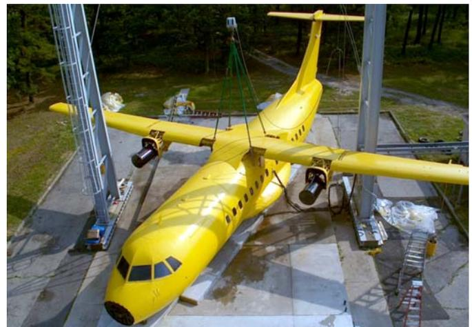
FIGURE 4. FUSELAGE TEST SECTION ATR 42
