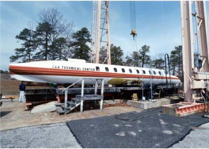
FIGURE 1. FUSELAGE TEST SECTION METRO III
