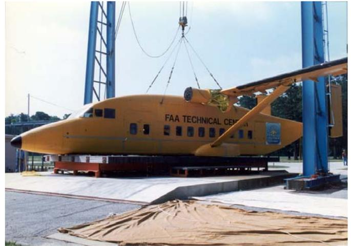
FIGURE 3. FUSELAGE TEST SECTION SHORTS 3-30
