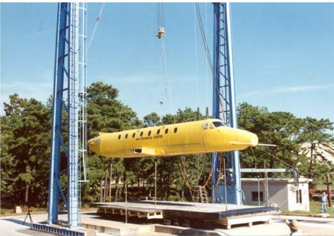
FIGURE 2. FUSELAGE TEST SECTION BEECH 1900C
