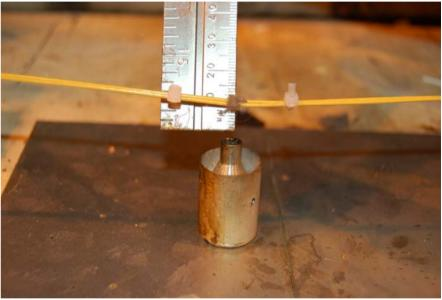
For the pristine samples the flame was applied for over 10 minutes with no arc over
