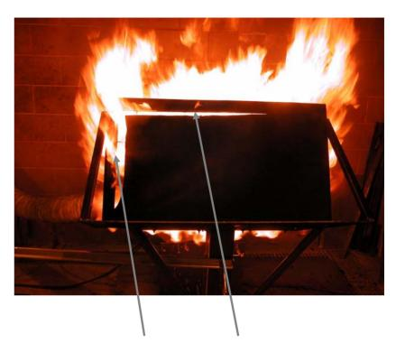
Material will typically shrink within 20 sec. from the top and the sides. The center portion, where the burnthrough is occurring, will not be affected by this.
