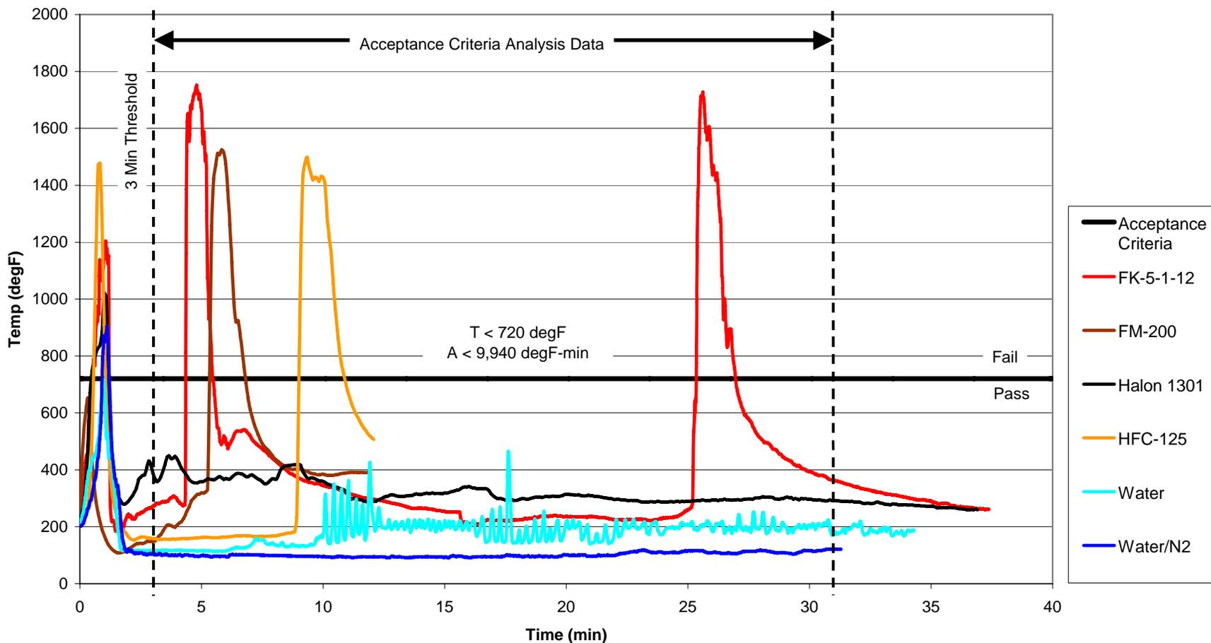
Fire Extinguishing Agents Tested Using the Aircraft Cargo
