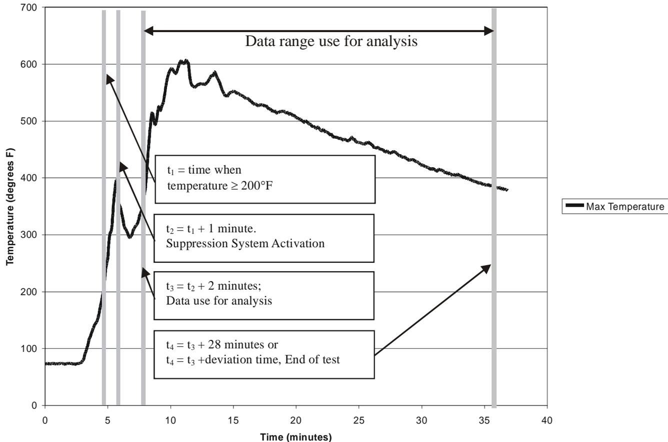
For Bulk Load, Containerized, Surface Burn Tests Only
