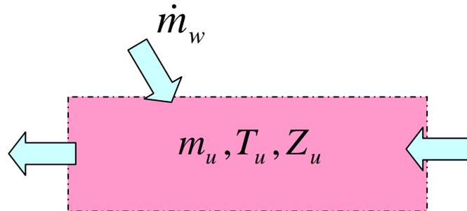
$$\frac{dT_u}{dt} = \frac{\dot{Q}_{fire} - \dot{Q}_{water}}{(m_u + m_{evaporated})c_p}$$
