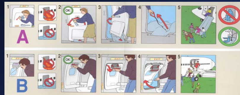
Pictogram A presents operating instructions for a floor-level exit and pictogram B presents operating instructions for an overwing exit.
