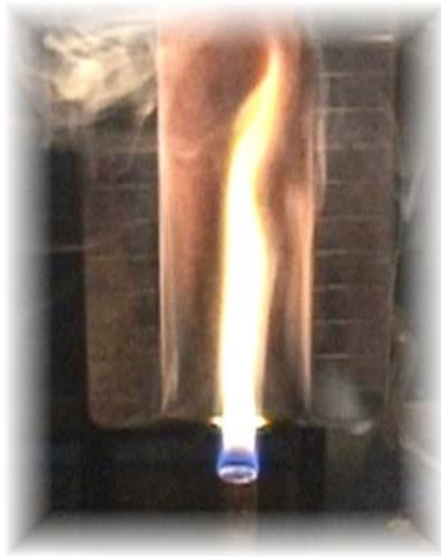
Vertical Bunsen Burner Test
