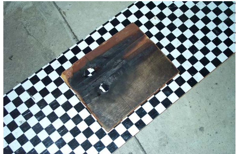
Tested at 1BTU/ft 2 Radiant Heat
