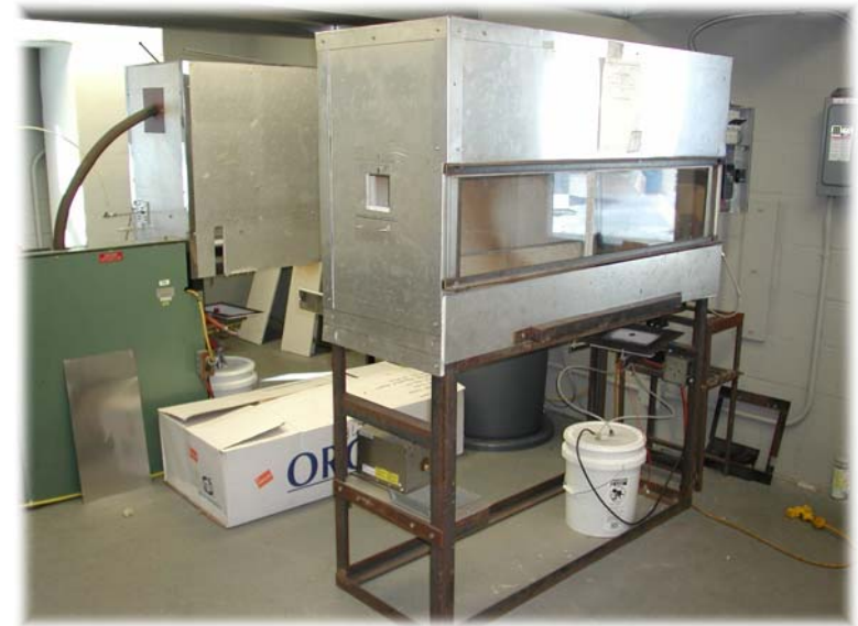
Radiant Heat Panel Test Apparatus (same as FAR 25.856)
