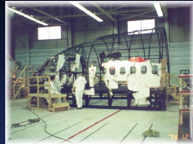
SwissAir MD-11 Accident Investigation Reconstruction, 1998
