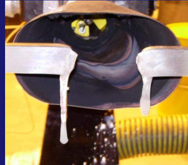
Part 2 Seat Cushion test used as severe condition for preliminary Mg Alloy data.
