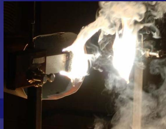
AZ31 - Burned when melted
