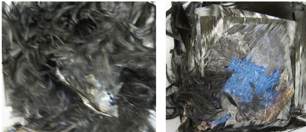
FIGURE 19F. AFTER BURNING FRONT AND BACK, 85 \text{ kW/m}^2
