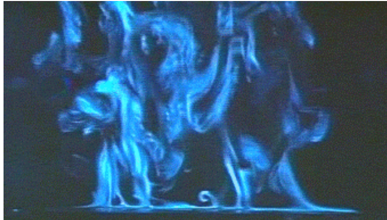
Figure 7. Growth of vortical structures from the surface of a heated flat plate
