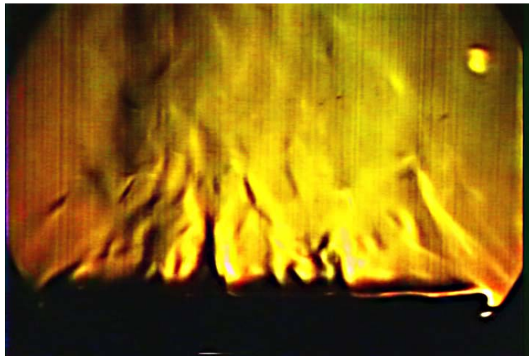
Figure 6. Schlieren Image of the flow field over a heated circular flat plate
