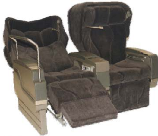
Figure 8. Passenger seat with a horizontal bar on an armrest (SICMA)
