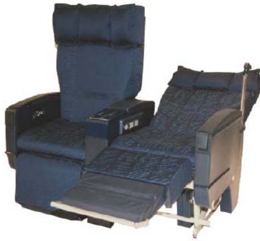
Figure 7. Passenger seat with a vertical bar behind an armrest (SICMA)
