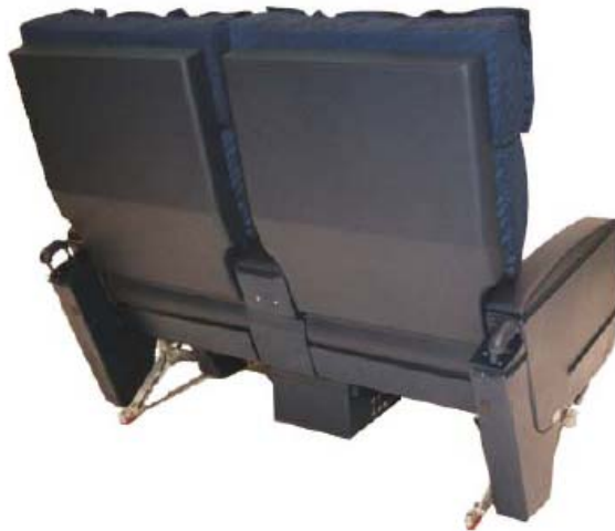
Figure 9. Passenger seat with a handgrip behind an armrest (SICMA)
