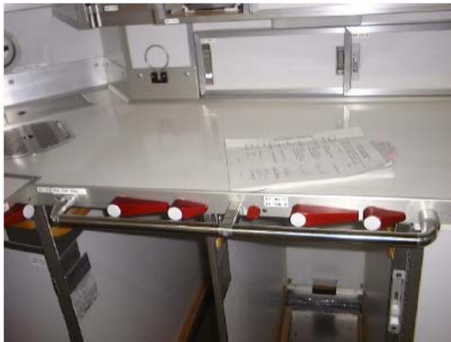
Figure 15. Improved handholds in a galley
