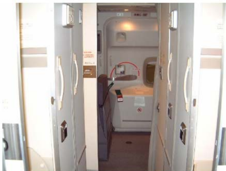
Figure 13. The suitcase handle equipped on the toilet outer wall
