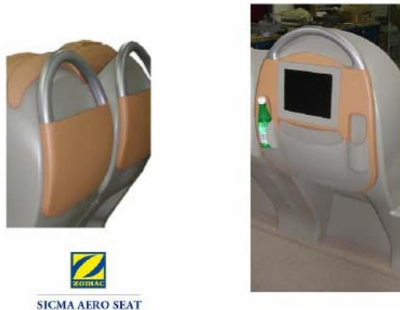
Figure 10. Passenger seat with a handgrip on the backshell (SICMA)
