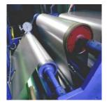
Cogebi developed an original process for the manufacture of very thin mica paper. The choice of a high particle diameter to thickness ratio, combined to the formation of a continuous sheet allows the self-orientation of the particles. That guaranties the best flame barrier behavior that mica can exhibit. A pure mica paper of  $25 \text{ g/m}^2$  is already an excellent flame barrier.
