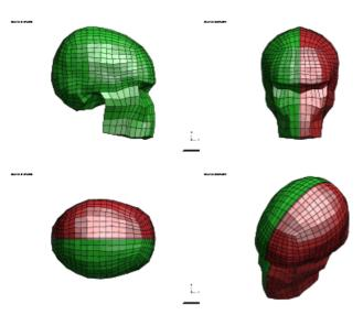
The Taleb model was adjusted to achieve comparative results between the ATD and the human model. However the approach was to adopt minimal changes and all default parameters were kept unchanged. The scale of the model was slightly increased to match the Hybrid III. The mass (Skull density) correlated well, with the human head 4.33 kG vs Hybrid III 4.40 kG. The center of gravity of the human head is 15 mm in front and 10 mm above the Hybrid III cg position.
