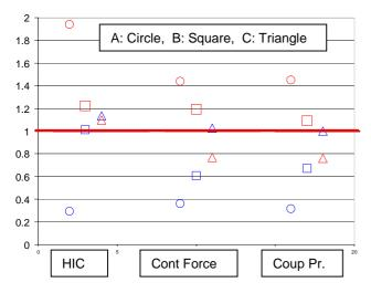
HIC as a predictor of injury correlates well with that of contact force or coup pressure, although at smaller impact pulses the results are more variable. Of the eight parametric runs, all three responses yielded the same pass/fail result. A correlation was made between HIC and contact force, and large population predicted results were generated. The pass / fail ratio was then compared to give a better estimate than only eight runs.
