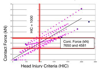
The results indicated that HIC reaches the threshold value of 1000 units at about 13G, where contact force, using a broad impactor crossed the threshold of 7650 kN at about 15 G. The correlation of pass/fail ratio for contact
