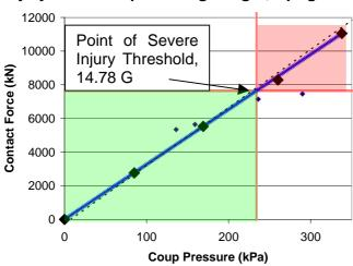
The large black diamonds show the experiment points for the factors B and C set to 10% Slack and Upright, while Factor A varies from 12 to 16 G's. The blue line is the predicted response between the test points. The small diamonds are the test points at other factor levels, and dashed line is the trend line for the correlation.
