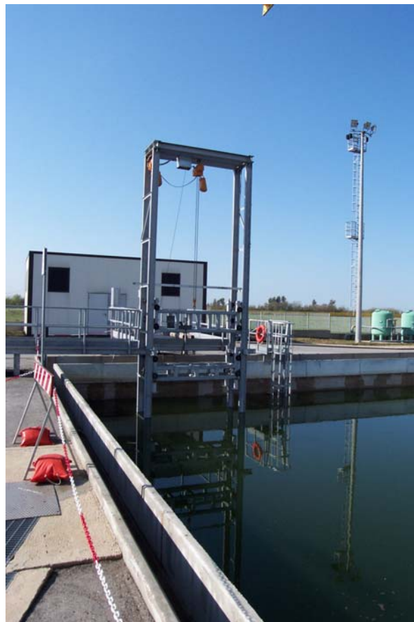
The guided drop tower at one corner of the pool (11,5 m high)
