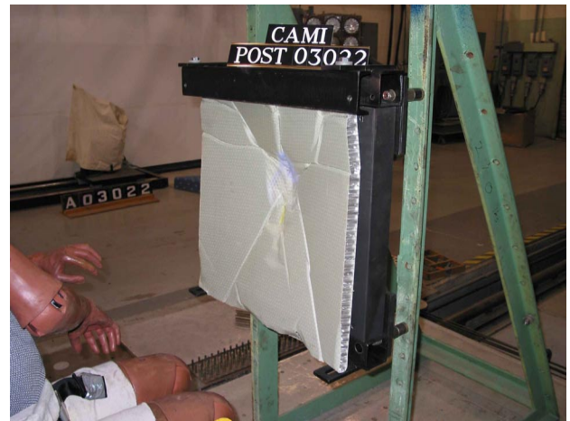
Figure 9. Aluminum Honeycomb Post-Test
