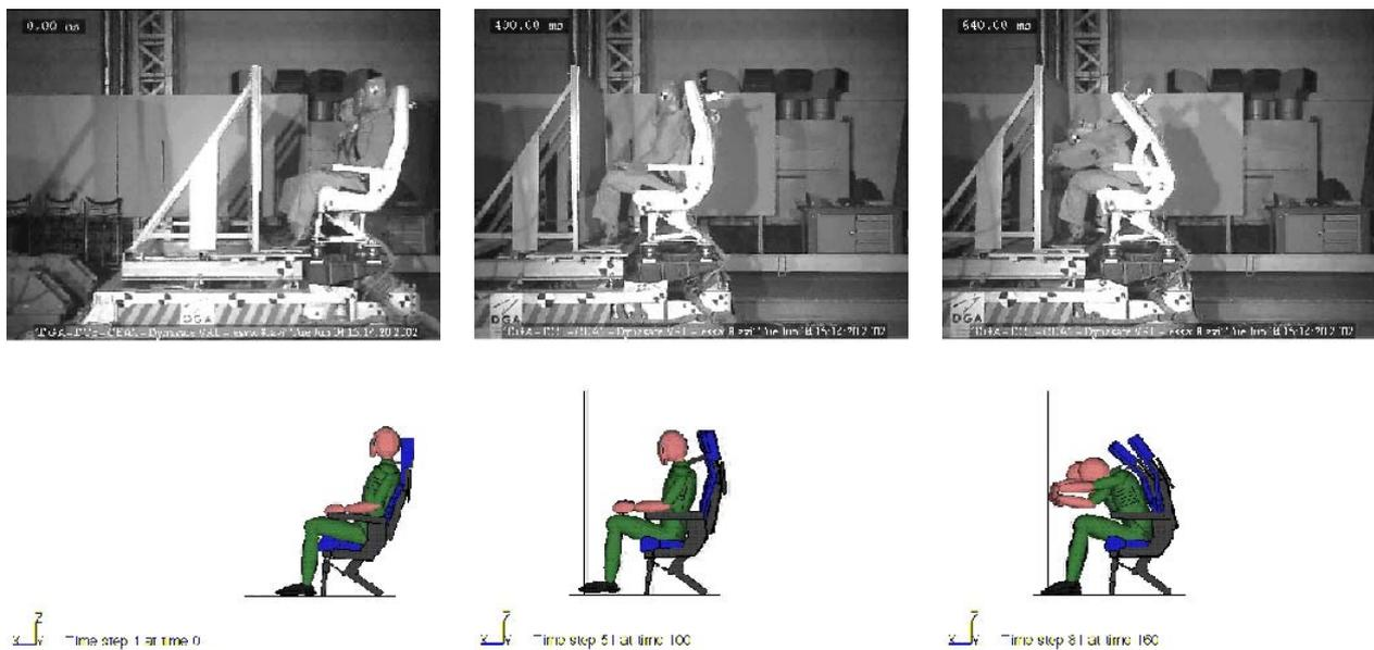
**Figure 2: MADYMO model versus horizontal 16G bulkhead test kinematical correlation (Left: Time: 0ms, Middle: Time 100ms, Right: Time 160ms)**
