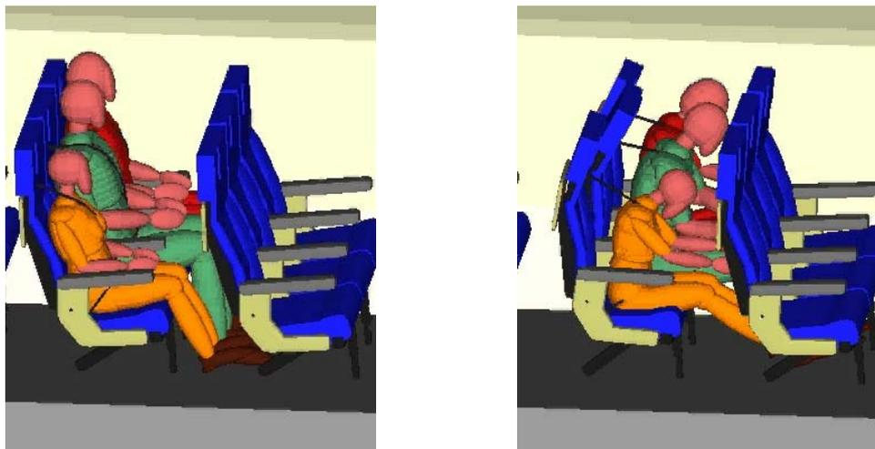
**Figure 7: Row to row simulation: 5%ile aisle (near), 95%ile mid, 50%ile window (far)
