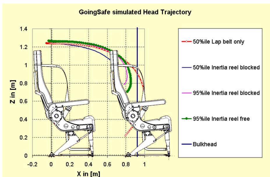
**Figure 5: Head trajectories projected on a row to row configuration (32" pitch)**
