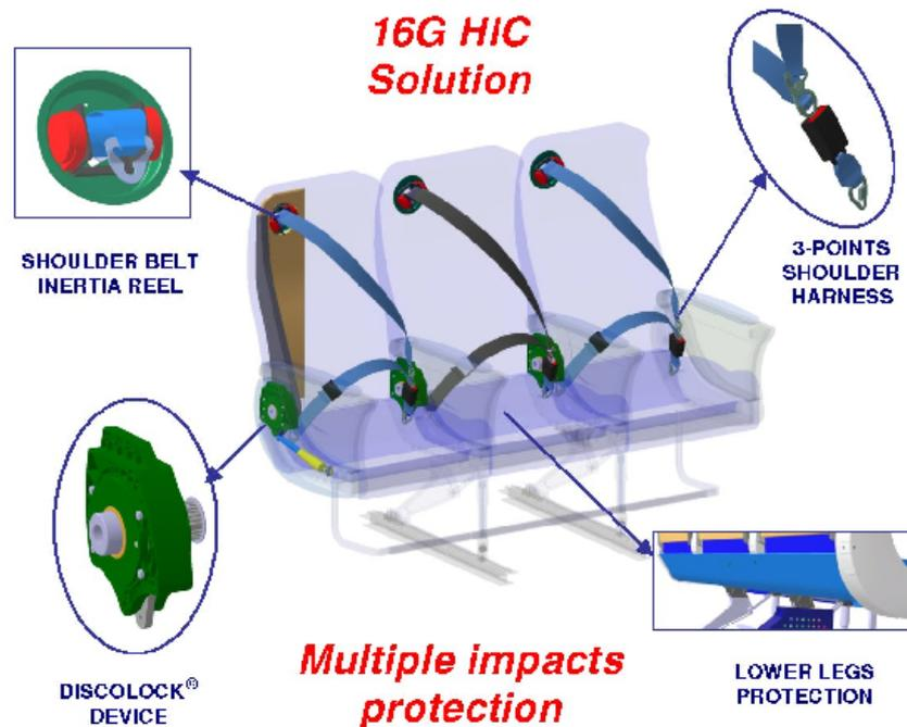
**Figure 8: GOING-SAFE triple seat design for A320 family**
