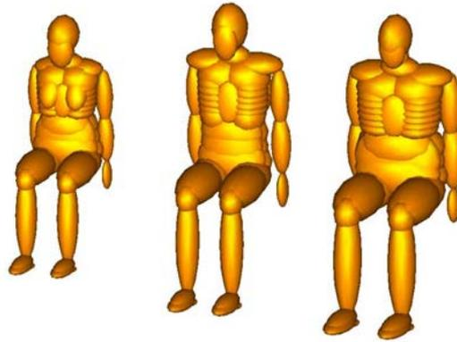
**Figure 3: Hybrid II dummy scaled models. Left: Small female (5%ile), Middle: Average male (50%ile, base for scaling), Right: Large male (95%ile)**
