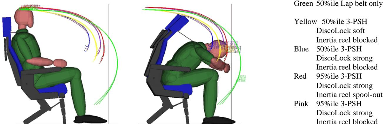
**Figure 4: Simulation with 95%ile occupant in front row configuration (Bulkhead on 920 mm from rear leg tie-down point)**
