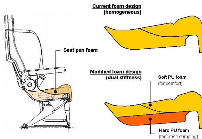
**Figure 6: Dual-stiffness-foam concept combination of comfort and crash damping**
